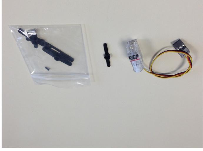
In the first step please prepare the servo by dismount the servo- lever/cross and the screw fixing it. The screw will not be mounted again later. For our small (micro) valves another servo-lever is needed (see picture below)
