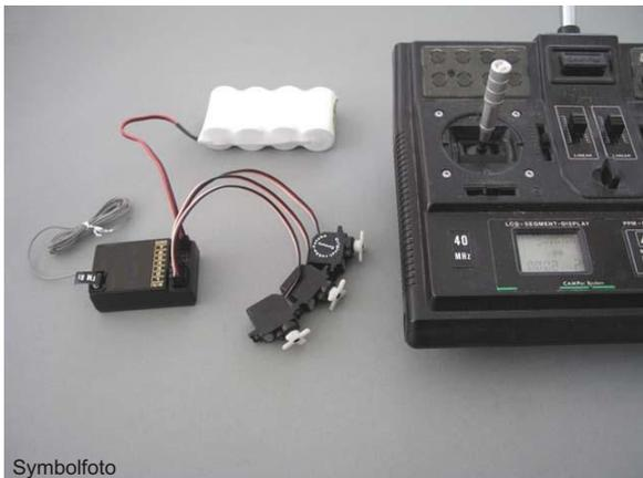
By the transport or dismounting the lever/cross from the servo it is no longer in a defined position. So **before mounting** it into the valve you must once connect each servo to the corresponding output-channel from the receiver of your remote-control-unit with which you later want to control the hydraulic function.
